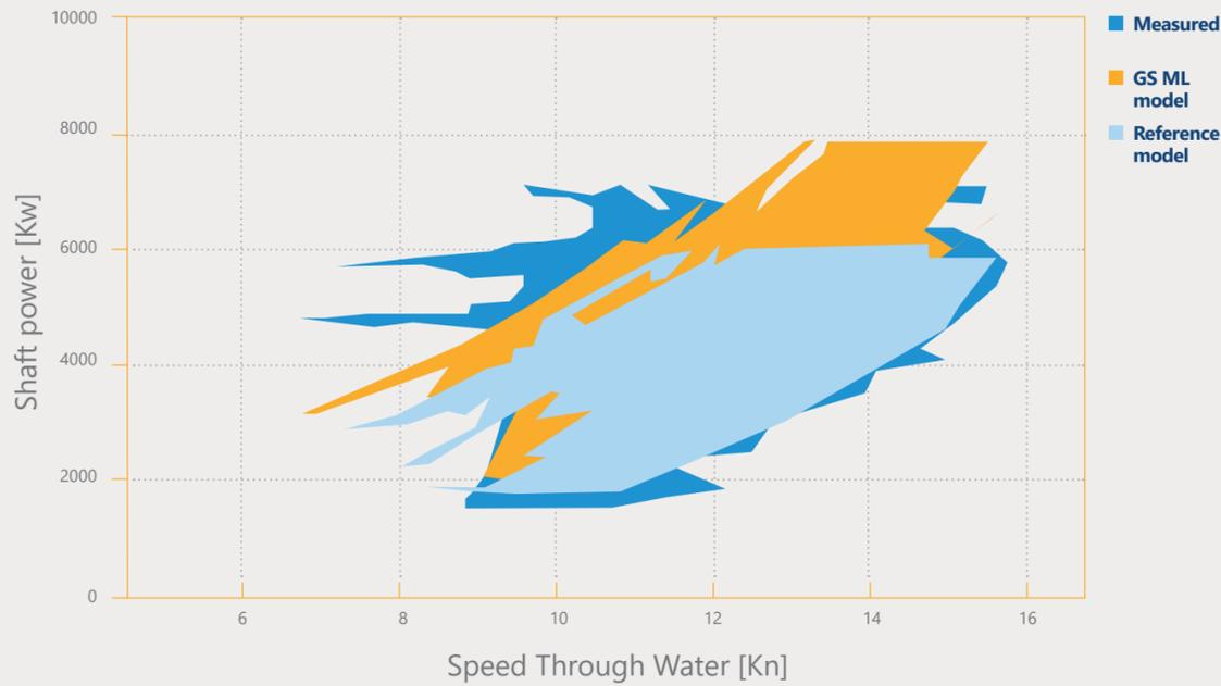
The optimisation process is sensitive to the shaft power and fuel consumption prediction, and therefore different models may produce significantly different speed advice. The **voyage route** is shown in the second image.
