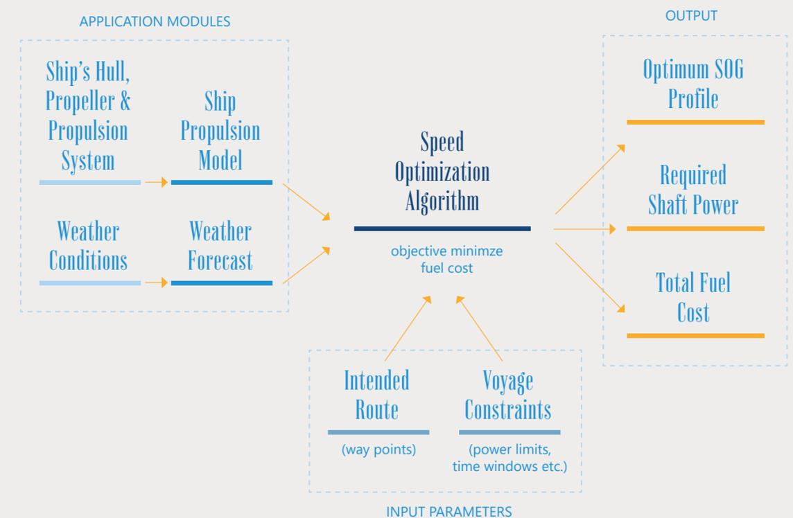
**GreenSteam Speed Optimisation** utilises a state-of-the-art, in-house developed **Hybrid model that harnesses Machine Learning and Operational Data (Big Data)** to achieve higher prediction accuracy by learning from the data.
